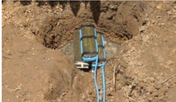
Figure 83: a combination of Anti-tank and C4 to be exploded Under the tiller system
