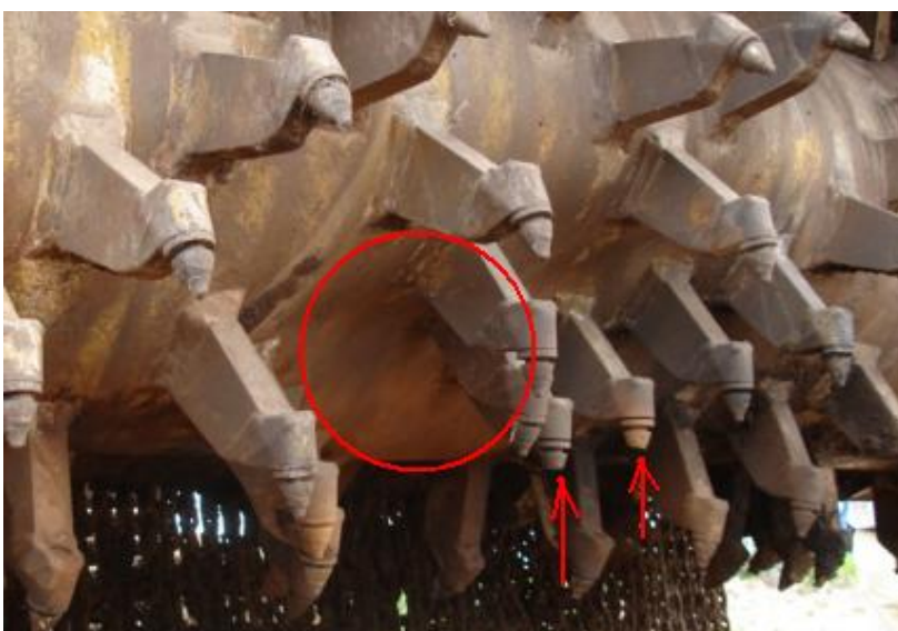
Figure 112: broken pits and a hollow drum
