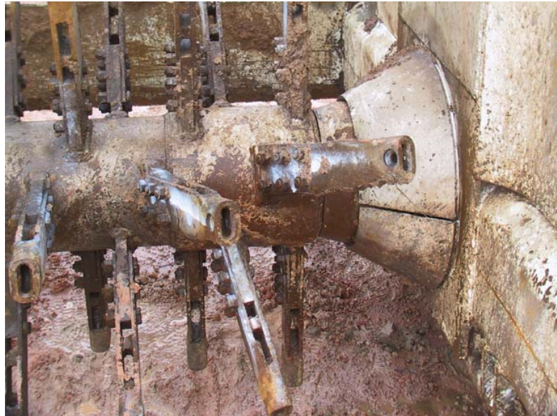
Figure 108: Holder are bending by Anti-tank blast
