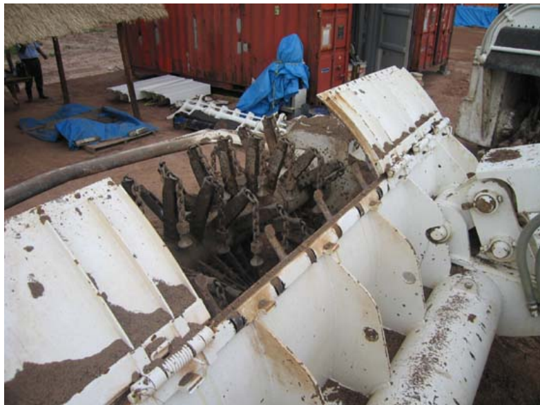
Figure 109: Anti-blast upper plate are blown away by Anti-tank blast
