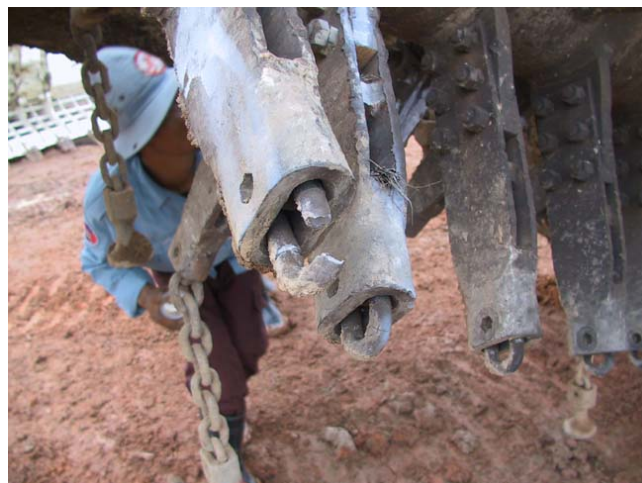
Figure 107: Chains are broken by Anti-tank blast
