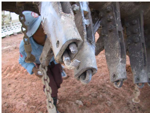
Figure 114: Chains are broken from Anti-tank blast
