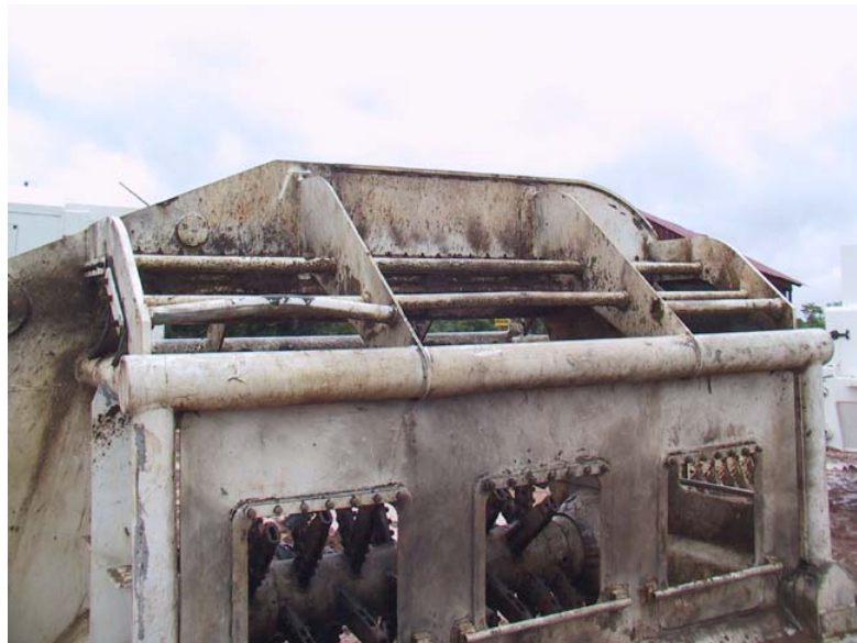
Figure 116: Rubber plate to protect dust are blown away by Anti-tank blast
