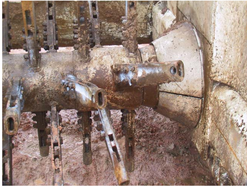
Figure 115: Holders are bending from Anti-tank blast
