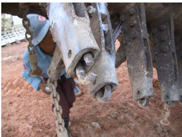
Figure 114: Chains are broken from Anti-tank blast
