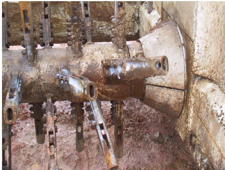
Figure 115: Holders are bending from Anti-tank blast
