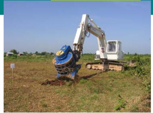
this Phase, the three demining machines were put in operational trials to assess their operational capabilities after modifications made based on the Phase I recommendations and further develop the SOP's for the demining machines.
